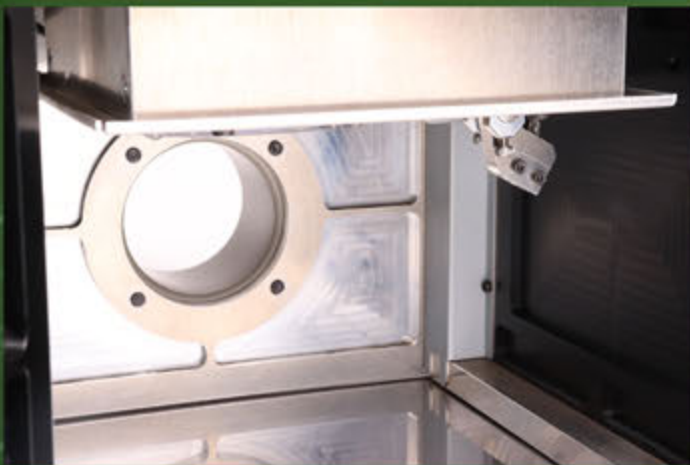
A guide laser for easy focus alignment.
